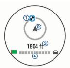
The destination indicator ① shows the direction of your destination relative to the direction you are moving ②. When the destination indicator appears at the top of the circle, you are heading towards your destination. The remaining distance to your destination ③ appears below the circle. The progress bar ④ shows your progress towards your destination.
