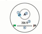
The destination indicator ① shows the direction of your destination relative to the direction you are moving ②. When the destination indicator appears at the top of the circle, you are heading towards your destination. The remaining distance to your destination ③ appears below the circle. The progress bar ④ shows your progress towards your destination.
